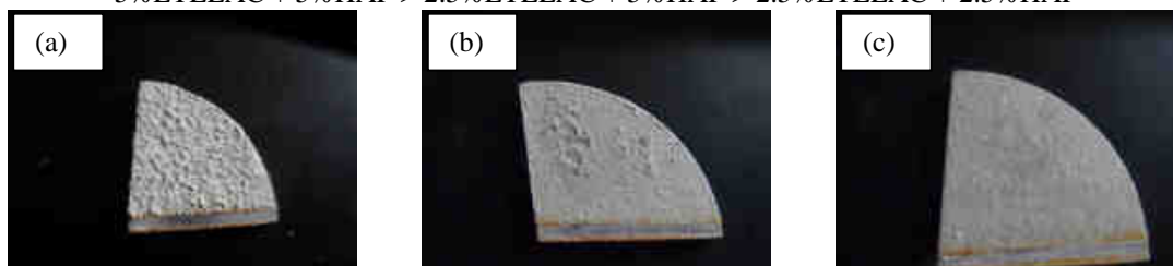
Fig. 6. Images of coated samples of M experiments using (a) 5 % ETELAC + 5 % HAP suspension, (b) 2.5 % ETELAC + 5 % HAP suspension and (c) 2.5 % ETELAC + 2.5 % HAP suspension with stirring at 150 r.p.m
