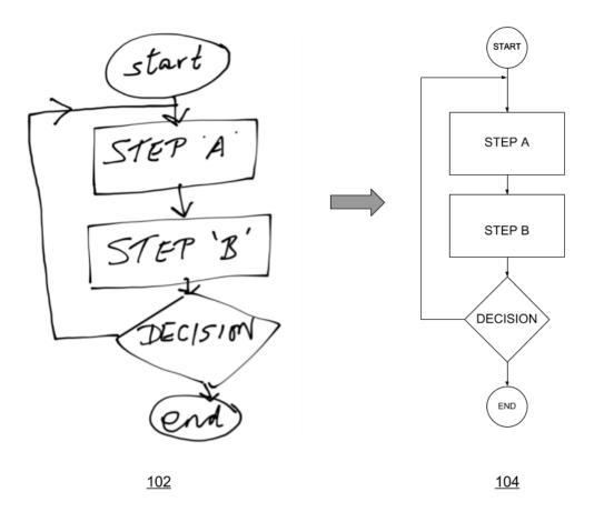
Fig. 1: A hand-drawn flowchart is transformed into a software-editable flowchart
