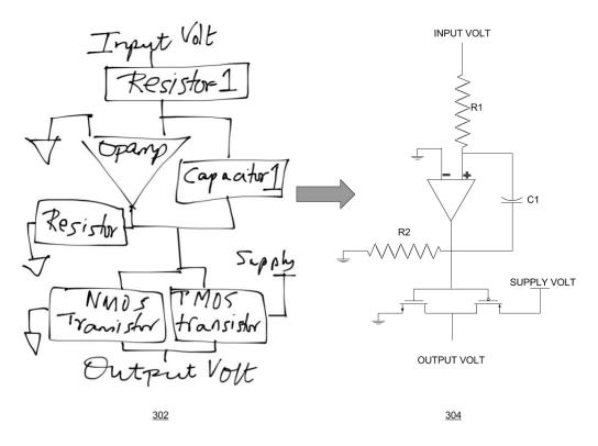
Fig. 3: A hand-drawn electronic schematic is transformed into a design-tool editable electronic
