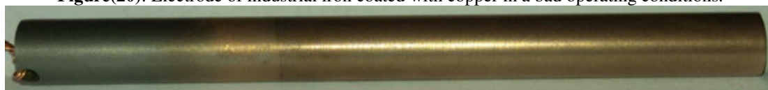
Figure(21): Electrode of industrial iron coated with copper in the appropriate operating conditions.
