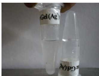
Figure (3): Thermally triggered release of liposome entrapped \text{Ca}^{2+} and formation of calcium cholate hydrogel doped with silver stable to tube inversion.
