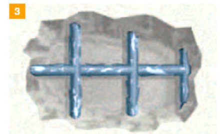
3 The salts reach the steel and dissolve the protective layer. Pitting corrosion starts to occur.
