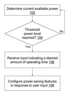
Fig. 1: Dynamic adjustment of power consumption based on time or event goals
