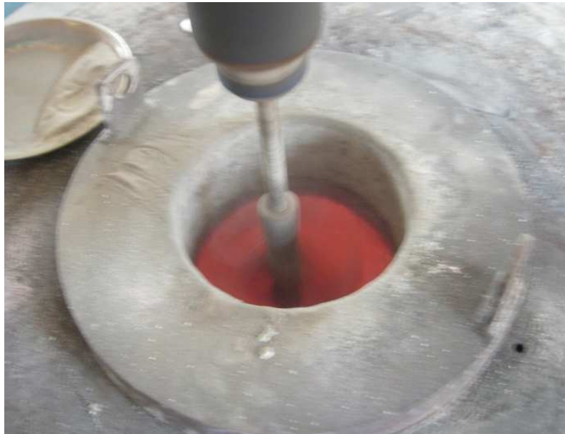
Figure 2: Close-up view of the stir-casting set-up. \text{Al}_2\text{O}_3 particulates of various sizes are added to the melt at 730^\circ\text{C} which is continuously stirred using a motorized stirrer made of ceramic coated stainless steel rod.
