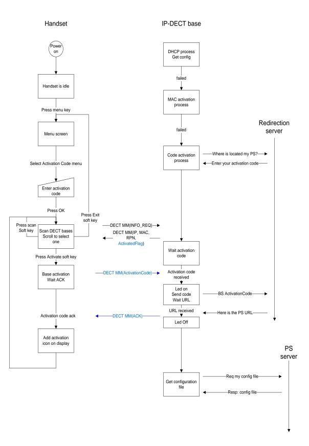
This above diagram on the left part shows the DECT algorithm in which the activation code is the same for all the DECT Base stations of the installation. For different activation codes, this algorithm has to be modified .
