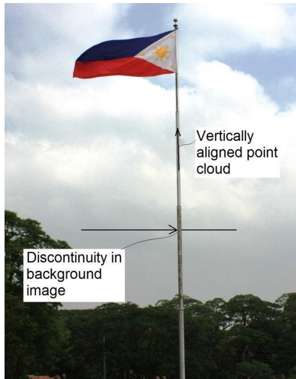
FIG. 1: Identifying thin objects in an image using image cues
