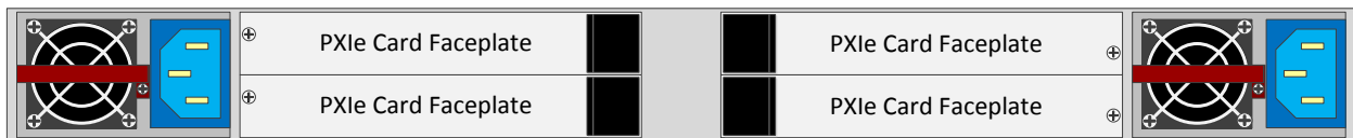
Figure 2. - 1U System with Four PXIe Cards, Chassis End View
