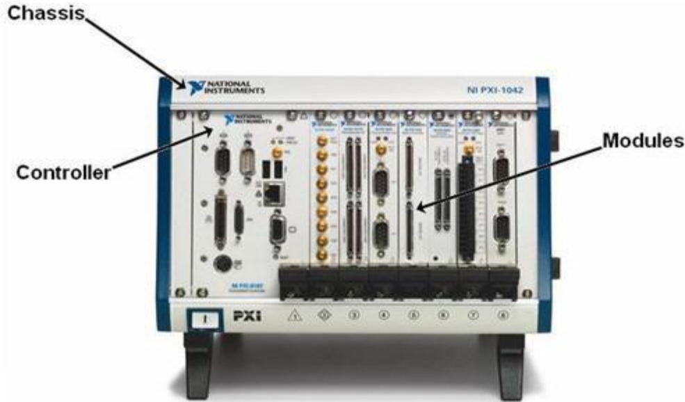
Figure 1. PXI system with 3U tall PXI cards installed.
