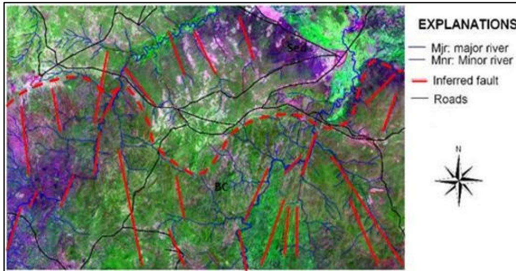
Figure 3: Landsat satellite image (1:50,000) and structural interpretation of project area showing dextral fault system. BC=Basement complex rocks. Sed=Sedimentary rocks
