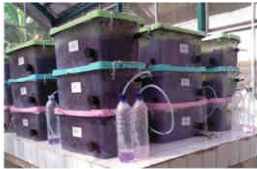
Figure 1. Bioremediation process using laboratory scale land-farming technique
