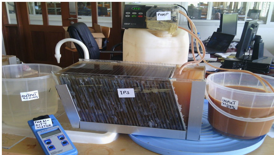
Plate1: Photo of the lab-scale IPS used in the experiment
