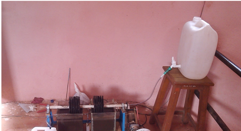
Fig 2: Lab Scale Set up of Two-Stage RBC
