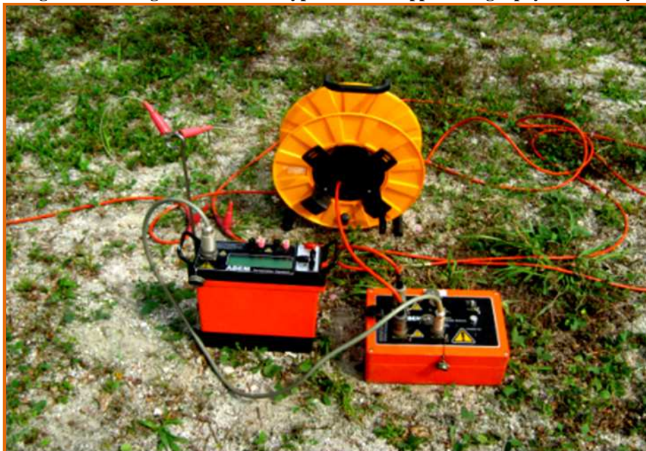
Figure 9: viewing the instrument type SAS1000 applied on geophysical survey
