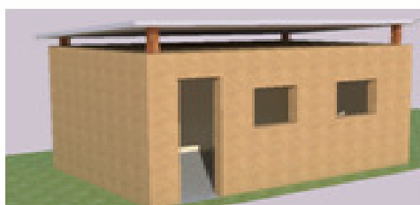
(a). Room with double roof
