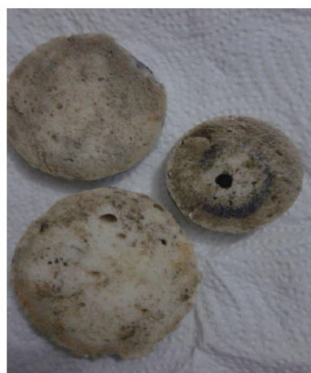
Fig(4c) Pu modified with peel garlic Burial in river soil
