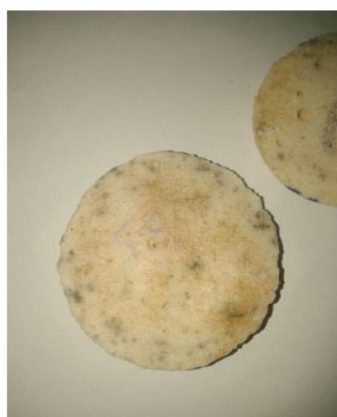
Fig(4b) Pu modified with peel garlic Burial in sand
