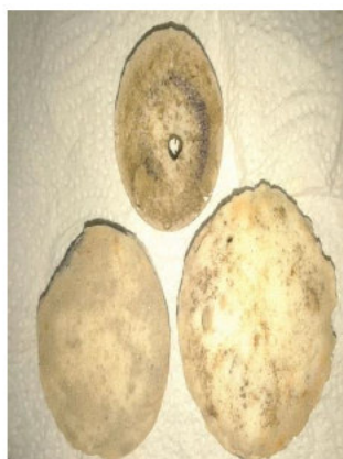
Fig(4a) Pu modified with peel garlic Burial in clay
