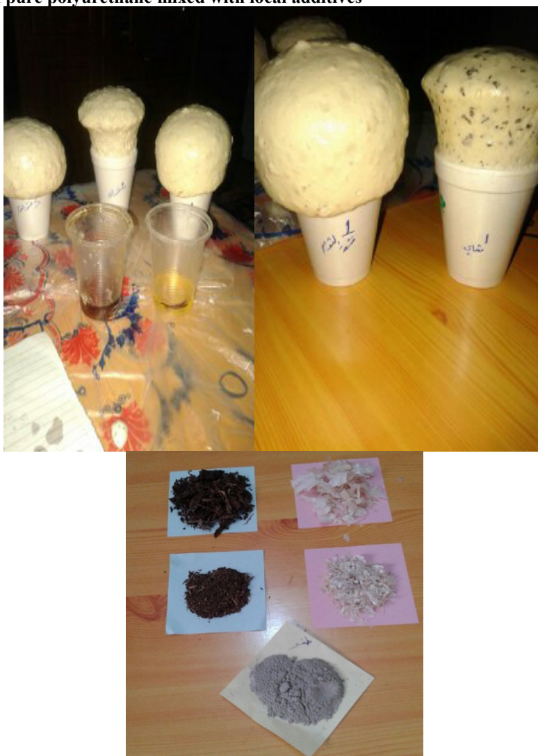
Fig. (3) Sample of polyurethane mixed with local additives
