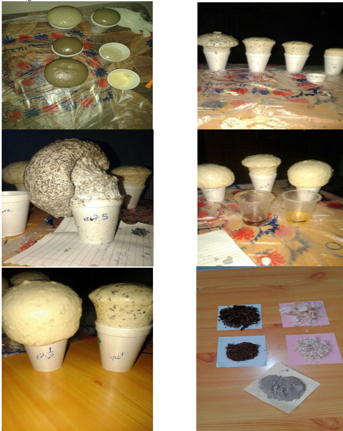
Figure(1) The modified polyurethane foam and the added materials
