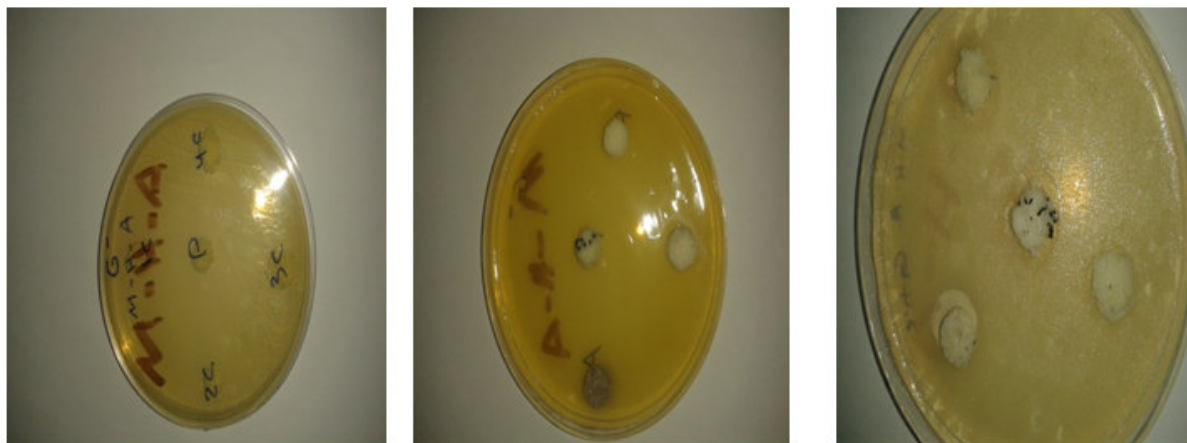
Figure(2): The modified polyurethane discs as antibacterial polymer
