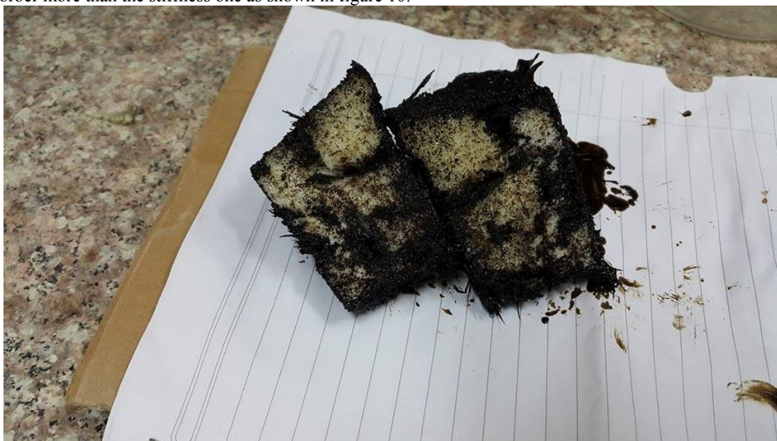
Figure 10. Polyurethane foam after the submerged oil.
