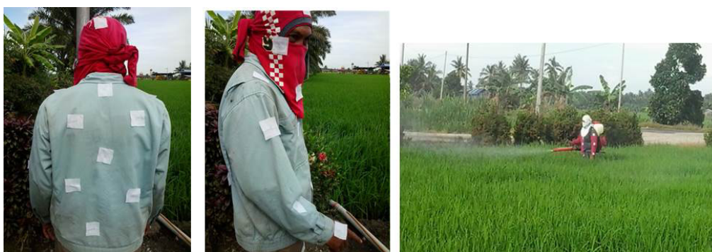
Figure 3. Spray operator was attached with cotton linens as showed in Figure (2) and perform the spraying activity as usual
