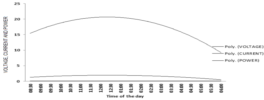
Figure7: Variations of polycrystalline current, voltage and power with time of the day
