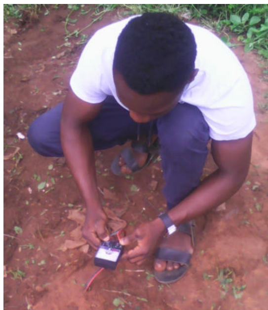
Plate 7: Soil moisture determination using Multimeter
