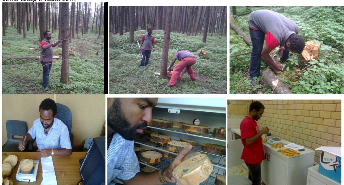
Fig. 2. From the top left to down right; measuring the diameter of the tree (DBH), felling the tree using chain saw, coding the harvested sample tree, weighting the sample disc by sensitive balance, removing the disc sample from the oven dry for checking, and measuring the dimensional change in wood specimens.
