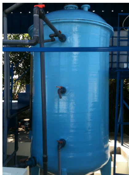
Fig 1: (A) Schematic diagram of RALBI: tank (1), peristaltic pump (2), decanter (3), up flow(4-5), Sampling point(wastewater, 6), Reactor outlet (effluent, 7) and Gas outlet(8) and (B): Picture of Reactor Anaerobic at Bacterial Bed Immersed (RALBI)
