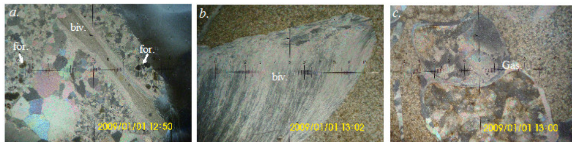
Fig. 3: Photomicrographs of limestones showing both laminated structures and recrystallization features. The laminated structures are well preserved on the bivalve (biv) fragments shown in (a and b). Although the foraminifera (for) shown in (a) exhibits recrystallization feature, this attribute is well displayed in (c), where a punctuated clear gastropod (Gas) fragment that appears at the center of the slide experiences partial and preferential replacement by microcrystalline calcite, with consequent destruction of the primary shell structure. In terms of mineralogy, calcite constitutes the most abundant mineral, while quartz and iron minerals are subordinate. In most of the thin sections, quartz grains are distributed interlocked with calcite. The calcite grains, which occur mostly in aggregate, comprises predominantly of medium- to coarse-grained, rounded to subrounded equigranular grains with few larger discrete spar occurring within matrix of very fine grained materials. The quartz show polycrystalline nature and sutured contacts under plane polarized light, which is indicative of partial recrystallization. Little or no flaky minerals or sulfide-bearing minerals occur.
