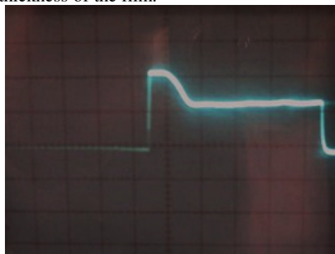
Fig.12. Image of the transmission of the laser beam when thermal lens is induced in VOPc doped PMMA film.
