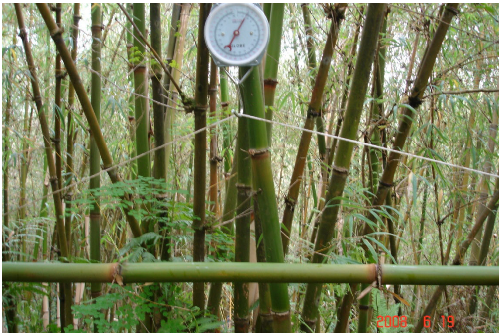
Figure 2. Measurement of green weight of bamboo culms
