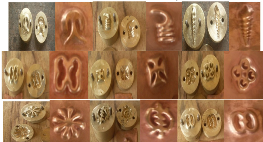
Fig.45: Die/punch sets and their bosses
