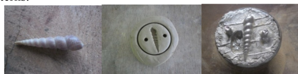
a: Pointed snail shell b: Clay mould c: Lead pattern
