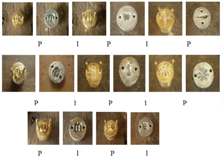
Fig. 39: Other punches and their lead dies
