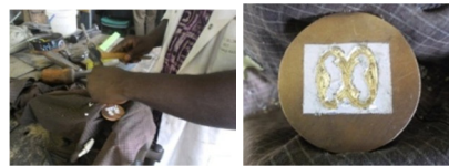
Fig. 20: Sinking of the die's models Fig. 21: Sinking of Nkonsonkonson symbol
