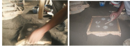
Fig. 28: Pressing and ramming processes Fig. 29: The finishing of the first mould
