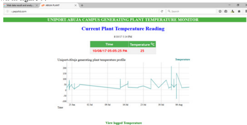
Figure 9: Captured Real Time Temperature profile
