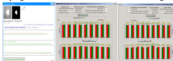
Figure 9. The results of the program in determining the center of the laser beam and its forecasting. The results of the program showed that the center of the image is determined by the laser beam profile and projected to the nearest pixel.
