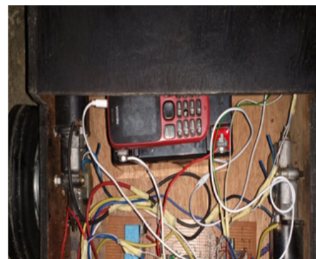
Fig 14: Fabricated GSM/RF based Robotic Circuit
