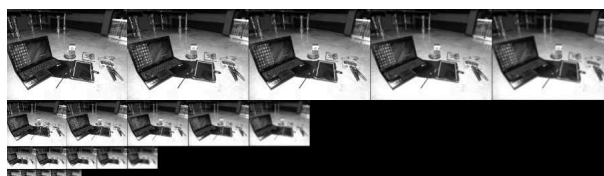
Figure 8. The pyramid of scaling of original image, scaled into four octaves of Gaussian filter, and each octave is scaled into five interval of dimension.
