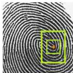
Figure 8 Core point (●) the region of interest, and window superimposed on a fingerprint
