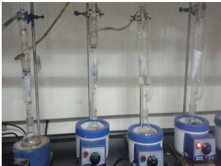
Fig. 8: Soxhlet extraction experiment for palm fruit fibre
