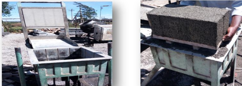
Figure 2: Point of reference for the design (multi-block-making-machine)
