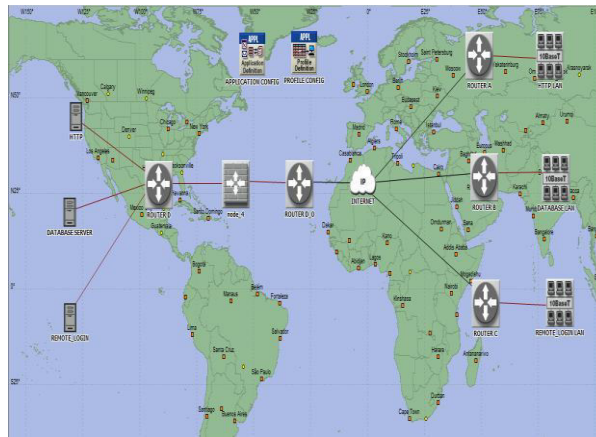
Fig. 3 Network Topology Using Firewall
