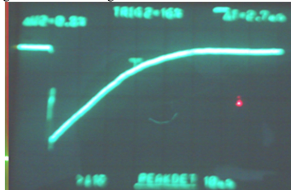
Figure (14) Voltage pulse for Marx generator- third stage 4.5kV.
