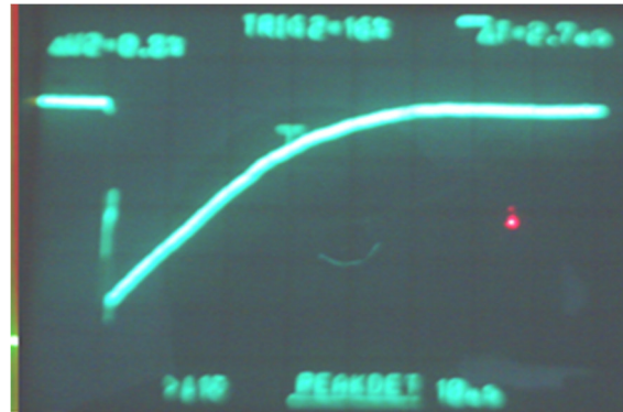
(b) Selected voltage pulse (first stage), Scale (1V, 10 μs)
