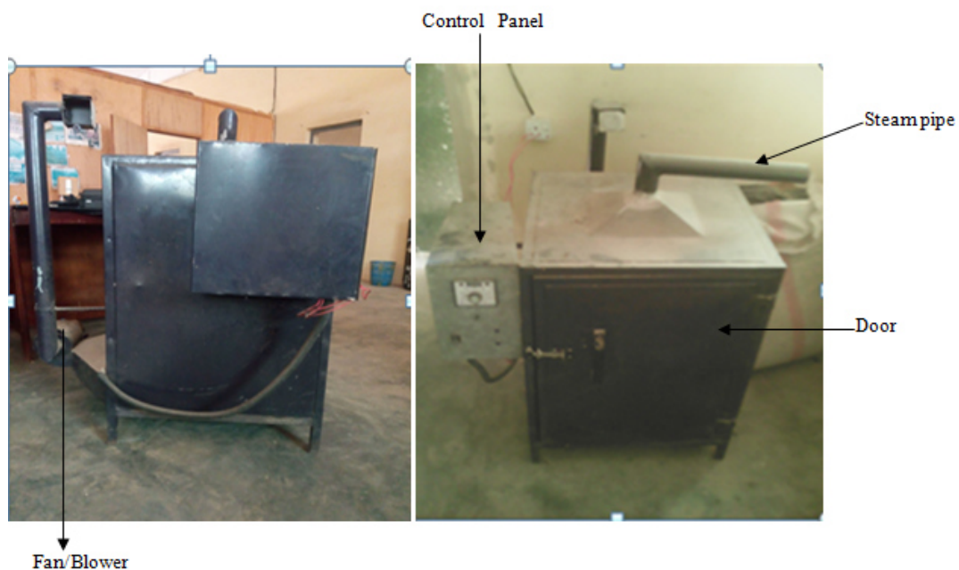
Figure 4: Pictorial views of the crop dryer
