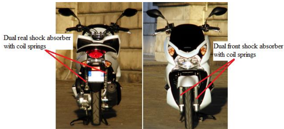
Figure 2. Dual rear and front suspensions of the SPX 125 scooter
