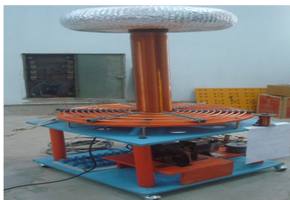
Fig.6.Complete setup of Tesla Coil.
