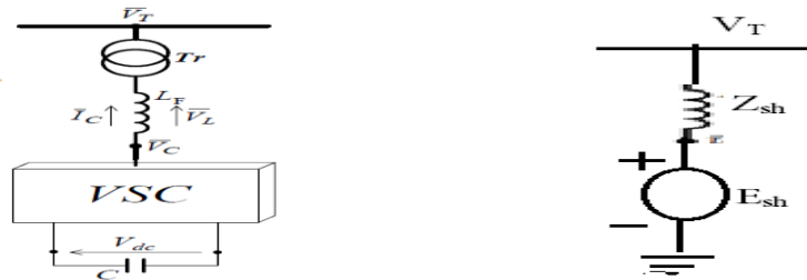
Figure 2 (a) STATCOM model construction (b) STATCOM representation
