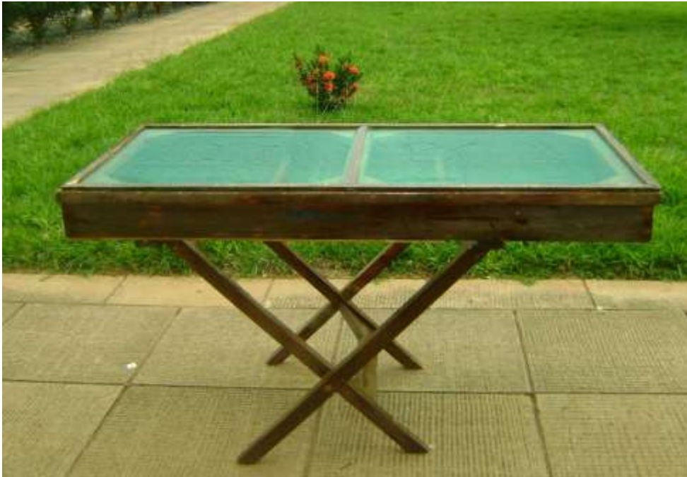
Figure 1: Simple box type solar dryer
