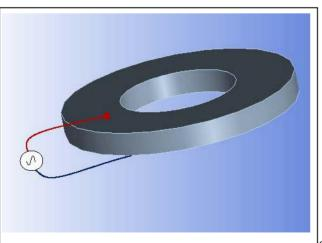
Figure 8: Electrodes connection on the piezoelectric ring.
