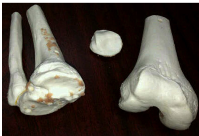
Fig.1: Gypsum is used as the material to produce the knee model in actual size obtained from a plastic knee.
