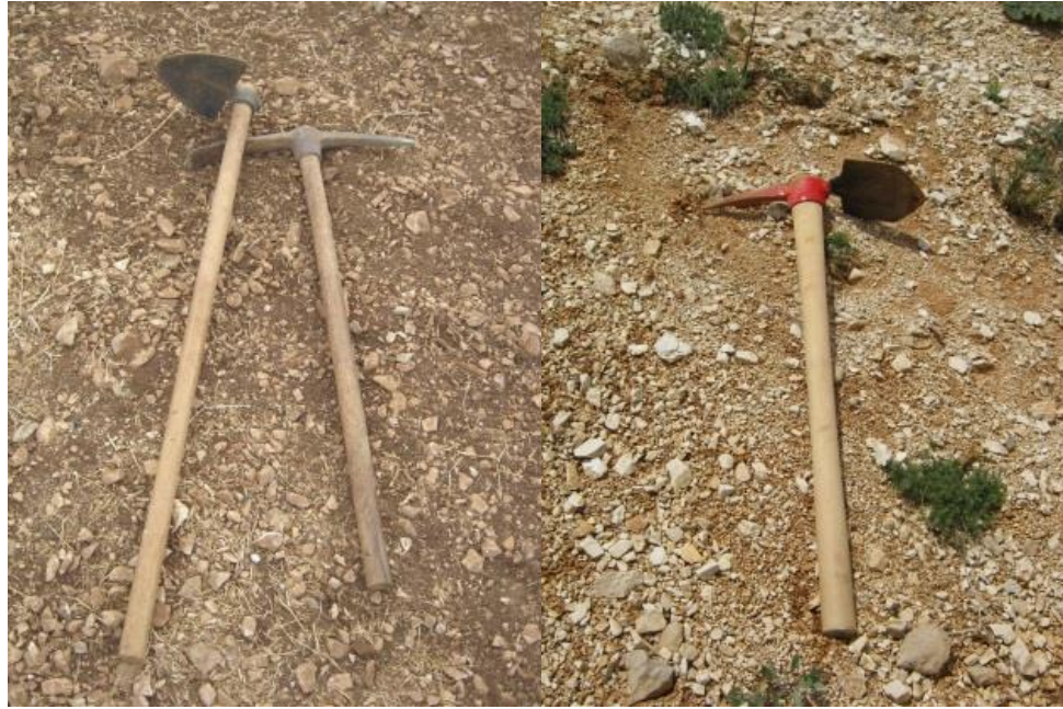
Figure 7. Left: Two tools, a hoe and a pick, were traditionally used to plant seedlings in Lebanon's rocky soils. Right: Combining them into a new tool has improved outplanting efficiency with reduced labor, and along with target plants, is increasing seedling survival and growth. Photos by Darin Stringer
