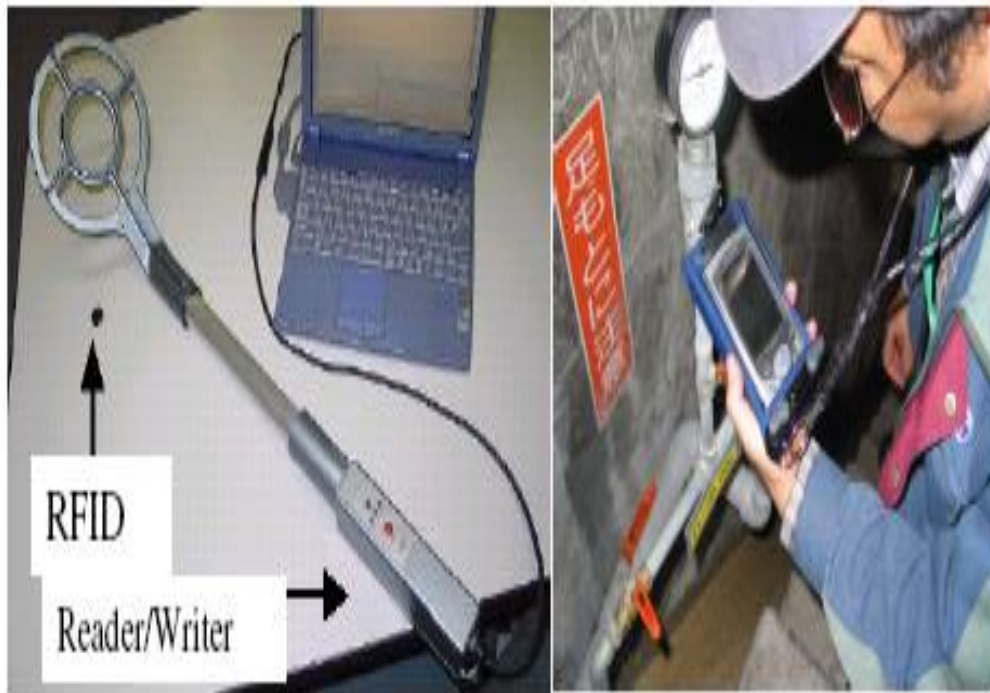
Figure 6. RFID and reader and a retrieving data activity by inspector from RFID by PDA (Yabuki et al., 2005)
