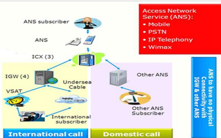
Fig 2: Call flow diagram of Domestic and International calls
