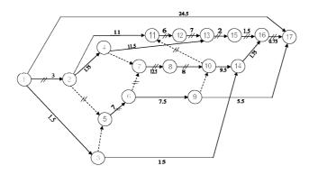
Fig.1 The mean of each activity is indicated on each arc and the critical path is shown in the network
