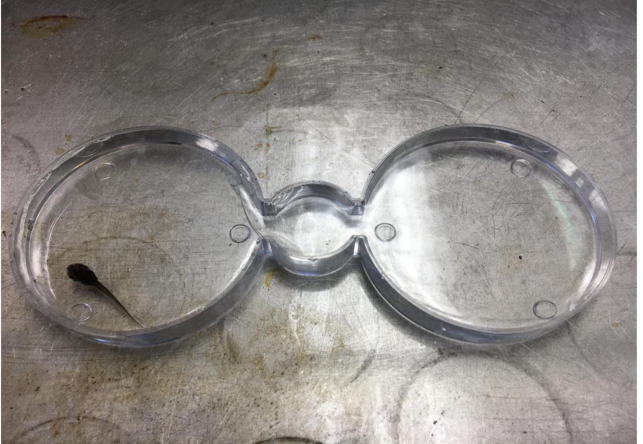
Figure 10. Wood frog tadpole choice trial arena. Dual 10 cm petri dishes with center connector.
