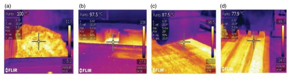
FIGURE 3. a) Delivery truck at the job site; b) Beginning of paving; c) Vibratory roller compaction; d) Pneumatic tyre roller compaction
