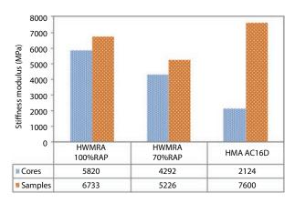
FIGURE 5. Stiffness modulus of laboratory specimens and cores
