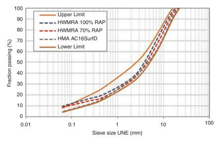
FIGURE 2. Gradation of the HWMRA and HMA mixtures
