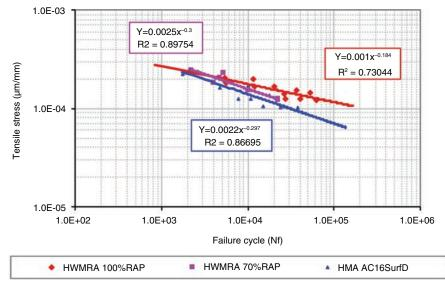
FIGURE 6. Fatigue limits of the cores
